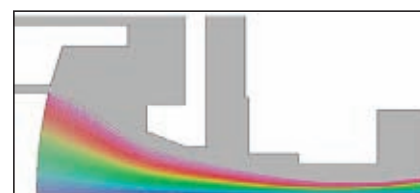
▲ Fig. 4 OPERA 2D finite element software—electron gun model.
